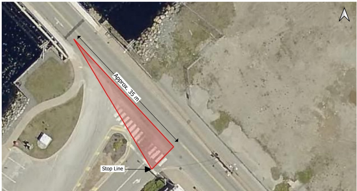
Figure 3-4: Intersection of Market Street and Henry Hensey Drive - EB Right Turn Lane
