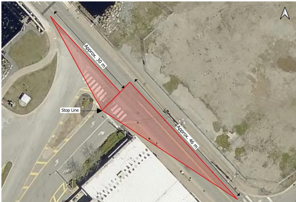
Figure 3-3: Intersection of Market Street and Henry Hensey Drive – EB Left Turn Lane
